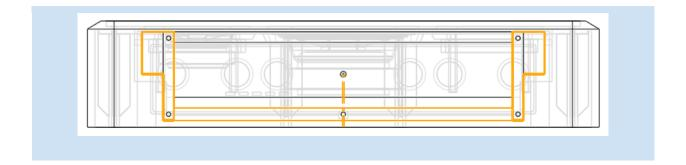
33. Now that we have the overall Frame shape defined, let's focus on the bottom side of the bluetooth speaker, where we will house the batteries and design a stand. Here is a picture of what we are going to sketch and extrude. Make sure to include the construction line in the middle. We will be referencing this line in week 8:
