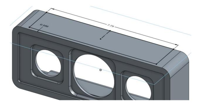
48. Extrude the profile downwards, and create a new part. Let's call the new part the "Button Overlay":
