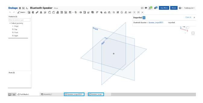
9. Let's delete the step file tab by right clicking, then Delete. We won't be needing the original file. We should now have a single, new tab, that shows the imported speaker geometry:
