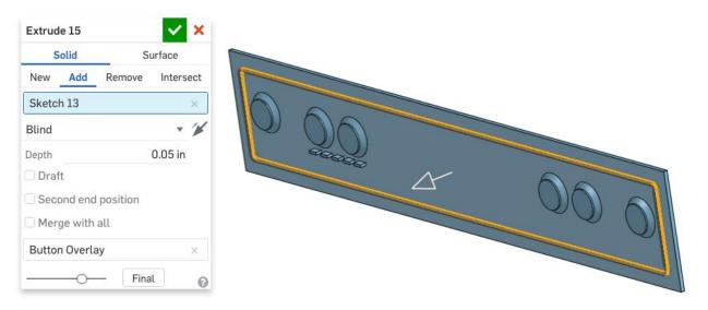
57. Next we are going to use all of this geometry that we just created in the Button overlay to remove material from the Frame using the Boolean Subtract tool, (1). In the dialog box, use the Button Overlay as the "Tool", and the Frame as the "Target". However, before we accept, check the "Offset" option, and select all vertical surfaces of the button overlays (highlighted below) and the LED overlays, and create a 0.01 offset. Make sure to "Keep tools":
