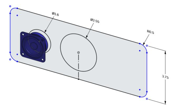
19. Next, add a dimension between the small circle and the outside edge of the housing (the small speaker has been removed for clarity):
