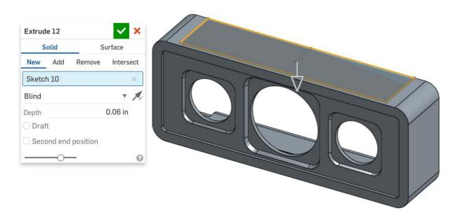
49. Hide the Frame part for clarity, and reorient to the "Top View" using the View Cube, as shown below. On the bottom side of the Overlay, sketch the circles for the buttons, again taking advantage of symmetry by using the sketch mirror tool.:
