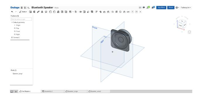
13. Notice how the speaker is not yet in the middle of our model. We know that the large speaker is in the center of the speaker enclosure, so it is best practice to move it there.
