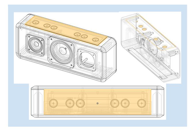
47. Next, we are going to focus on the top part of the Bluetooth Speaker, where the buttons go. Our design includes a soft rubber overlay that covers the buttons, for a nice resilient feel. Let's start by sketching the profile of the rubber overlay on the top of the Frame. The insert is centered about the origin, so we have used a construction line for creating constraints:
