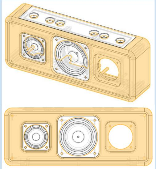
23. Next, let's extrude the entire sketch, holes and all, 2" deep symmetrical about the Front Plane. This should be a new part, and the small speaker may be hidden for clarity. The name of the new part is Frame:
