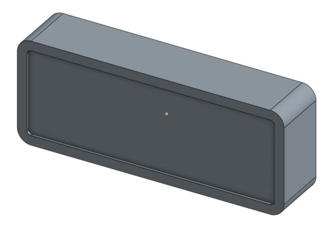
26. Next, use the same sketch to create a new part. Use the "Up to Face" option and select the inset face of the Frame. The name of this new part is Face. This is the front Face (or Bezel) of the speaker assembly.
