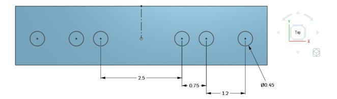
50. Now, extrude the buttons 0.1 in downwards. Make sure the extrude is added to the Button Overlay part:
