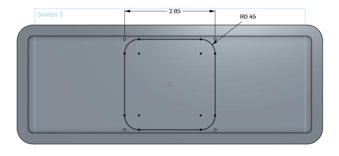
28. Now, let's use this to remove material into the Frame. It should be 0.15 in deep, and have 25 degrees of draft. Make sure the draft is in the right direction (there should be no undercut surfaces):
