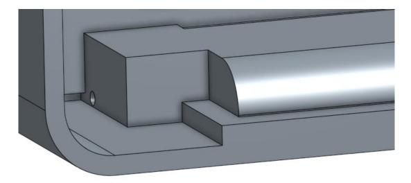
45. Next, we'll add the holes for the speakers. For this, we will reference our original sketch, and we will extrude it in two directions. First, we will extrude it "through all" towards the front of the Frame part. However, notice that the center hole interferes with our battery opening. This is because the extrusion "starts" at the sketch plane:
