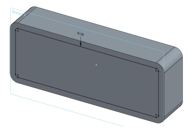
25. And let's extrude it 0.1" into the part, and remove material:
