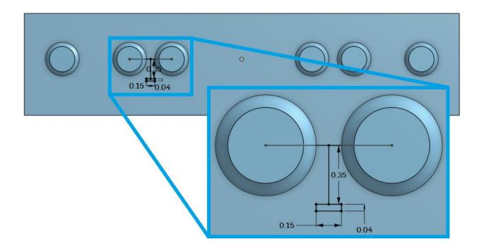
53. Now extrude the LED Overlay the same depth as the buttons (Hint: use the "Up to face" depth option). Note the orientation of the part below ,and make sure the LED overlay is in the proper location:
