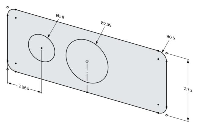
20. Next, since the part is symmetric, we can now use the vertical construction line to mirror the small circle over to the right. Start by selecting the Mirror tool, Lie. You will then be prompted by Onshape to select the sketch line to use for the mirror:
