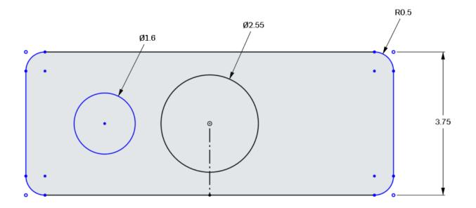
18. Now, let's constrain the small circle using the small speaker. To do this, unhide the speaker, and then use one of the circle edges on the speaker to create a concentric
