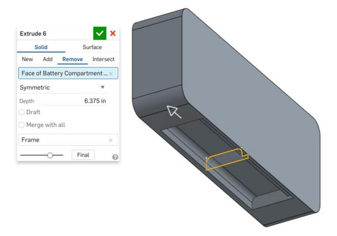
36. Now, let's add a relief on each side for the battery cover. Note that the sketch is symmetric (the construction line is used to mirror the sketch), and pay attention to the sketch plane, which is highlighted in orange:
