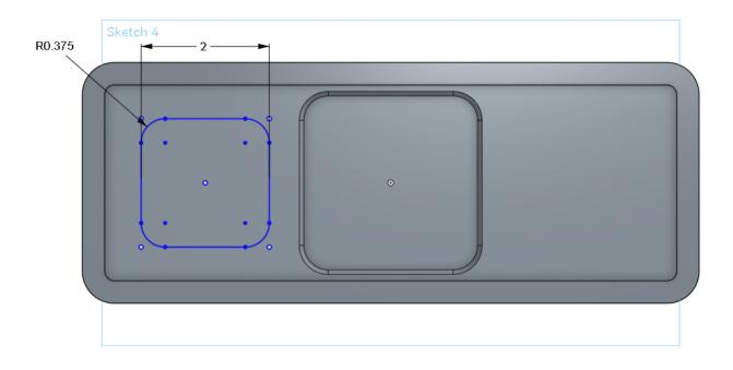
30. Let's locate our square using the circle from the first sketch. Unhide Sketch 1, and create a Coincident constraint between the center of the circle and the center of our square. It should lock in place, and turn black. Accept the sketch:
