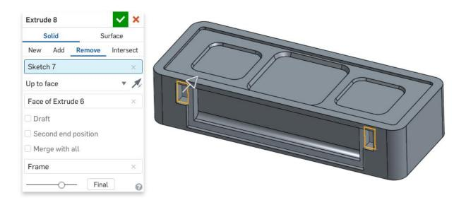
40. With the major geometry of the Frame built, we can now shell the part. Referencing the back face, create a 0.10 in shell. Imagine trying to do the job of Shell with just Extrudes!:
