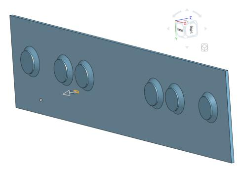
54. Now, we will create the rest of the LED overlays using a linear pattern. Use the edge of the part for the direction, and create a 0.25" pitch pattern in both directions:
