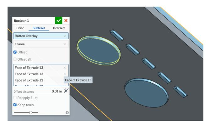
Pro Tip: What did we just do? Well, we just included an offset to the boolean subtract. This creates a gap between the parts. This gap will allow the lip in the Rubber Overlay to fit snugly into the frame, but without having the button and LED overlays interfere. This is important,
