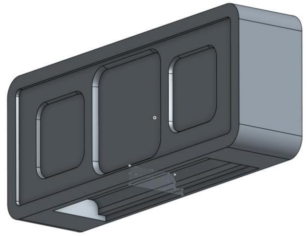
34. Start by creating the following sketch on the Right Plane. The outer dimensions (0.2, 0.125, 0.365, 0.14) are dimensioned from the outer faces of the Frame Part. Name this sketch "Battery Compartment Sketch":
