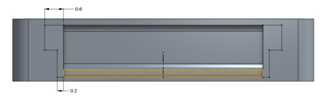
37. Using that sketch, remove material outwards Through All:
