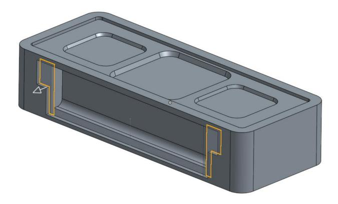
38. Next, using the most recent geometry as a reference, sketch two pockets on each side of the part:
